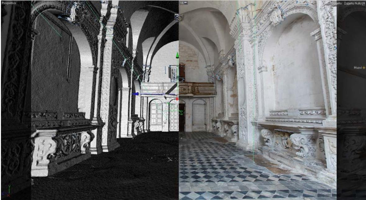
Figure 6: Screen shot of 3D model with and without texture applied.
